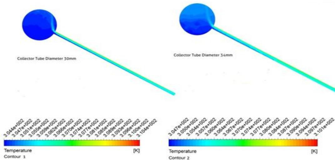
Figure 4.1 Contours of temperature for different diameter riser tubes after 4500 seconds, (a) collector tube diameter 30mm, (b) collector tube diameter 34mm
