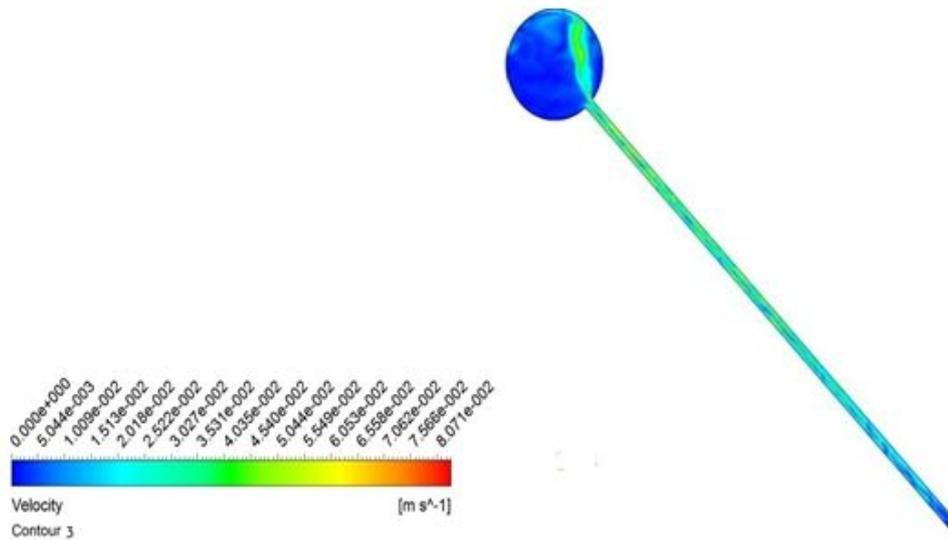
Figure 4.4 Contours of velocity for collector tube length 2m.
