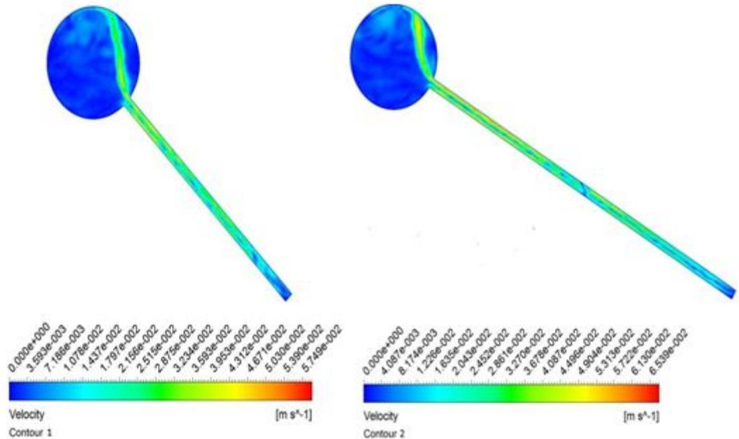
Figure 4.3 Contours of velocity for various tube lengths, (a) collector tube length 1m, (b) collector tube length 1.4m
