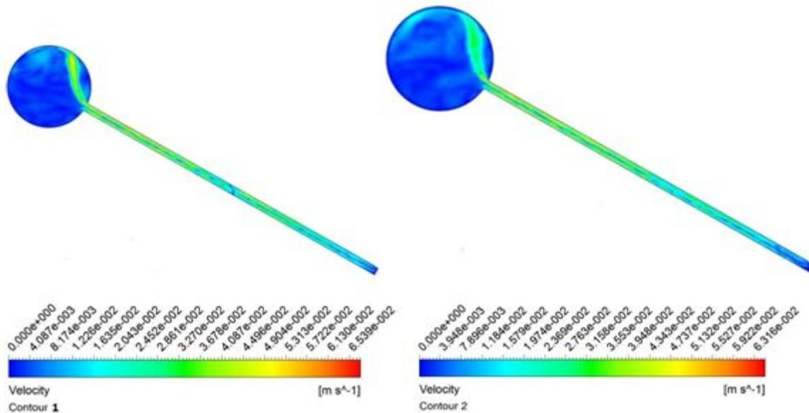
Figure 4.7 Contours of velocity for different tank diameters, (a) tank diameter 350mm, (b) tank diameter 400mm.
